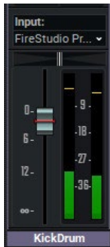
The volume (vertical) and pan (horizontal) sliders on a kick drum track.
