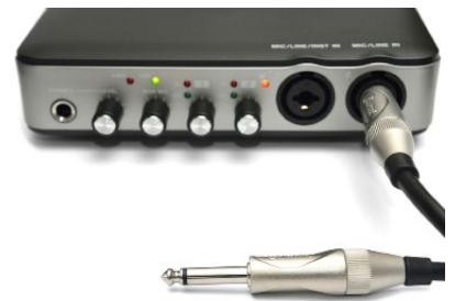
USB Audio/Computer Interface. This device supports the use of external microphones and instruments during recording.
