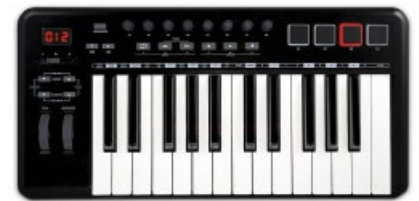
MIDI Keyboard Controller. Keyboards such as this model, work with Mixcraft and can play and control Mixcraft's built-in virtual instruments.
